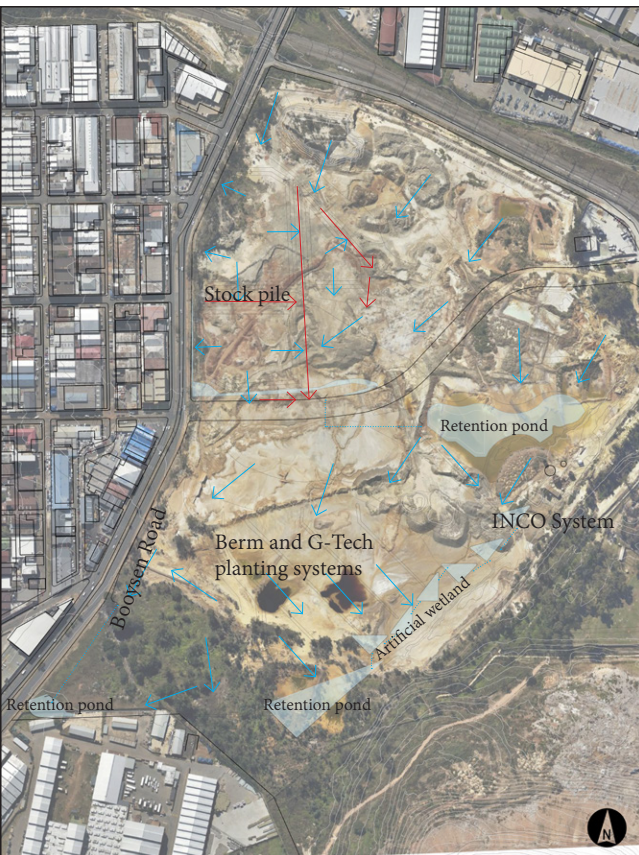
Figure 8.2 Phase one stormwater management (Author 2017)
