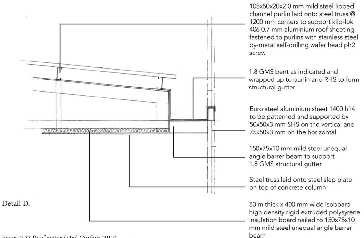
Figure 7.33 Roof gutter detail (Author 2017)
