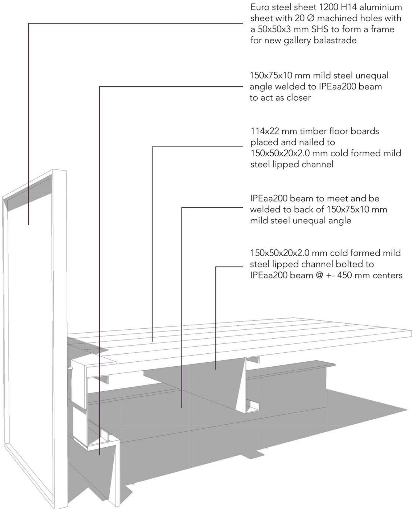
Euro steel sheet 1200 H14 aluminium sheet with 20 Ø machined holes with a 50x50x3 mm SHS to form a frame for new gallery balustrade
