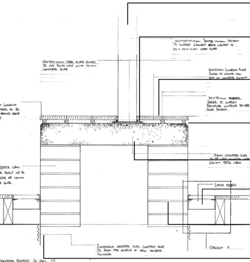
100x100x4.0 mm SHS to support gallery above welded to 120x120x10 mm steel plate
