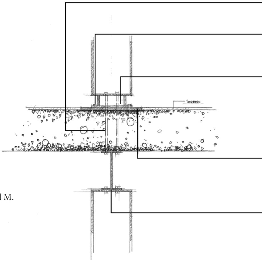
M12 rods cast into concrete floor to act as guides for accurate positioning of columns providing continuous connection to column below
