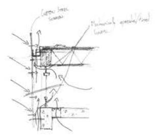
Aluminium Screen heated up preventing internal solar gain. Service walkway between screen and museum helps encourage ventilation pulling internal air through.
