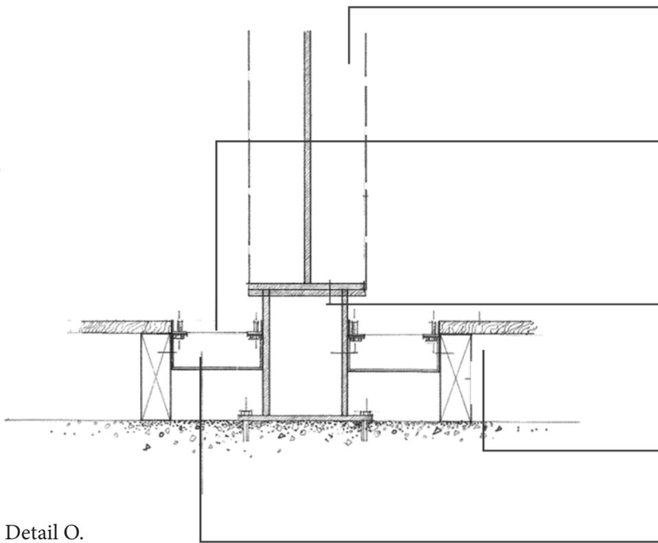
457x191x67 mm mild steel parallel flange I-section column to be welded to 457x191x10 mm steel flat
