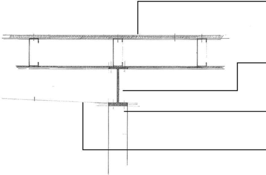
114x22 mm timber floor nailed and supported by 150x50x20x2.0 mm mild steel lipped channel @ 450 mm centers
