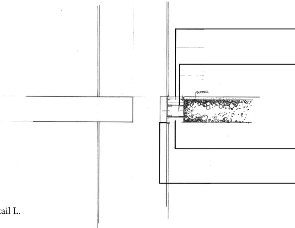
105x50x20x2.2 mm cold formed lipped channel capped with laminated glass held by 25x25x3 mm equal angle
