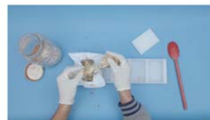
6. Remove mushroom mass from jar. Break into pieces and place into brick mould.
