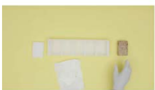
7. Remove the brick from the mould and wait for it to strengthen (1 week)
