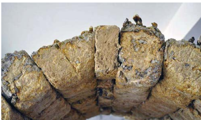
Fig 7.29 Mycelium bricks as building material (Mycoworks.com, 2017)
