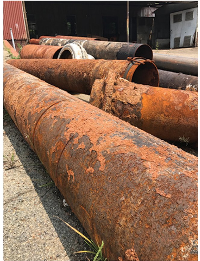
Fig 7.36. Reclaimed 450mm dia 'British Steel' round hollow tubes found on-site (Author, 2017)
