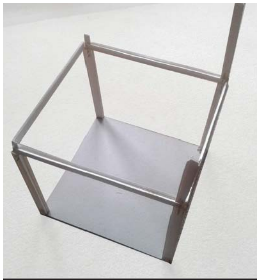
Figure 05.14.3 Model of structural iteration explaining the variety of uses and fixing of a single element for beam and column construction
