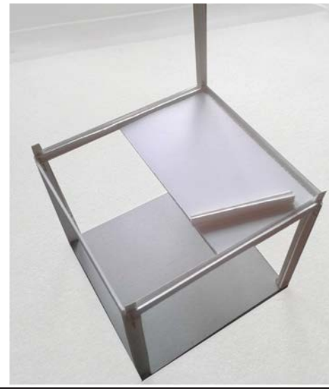
Figure 05.14.4 Slab cast between beam and quick assembly of structural elements for future adaptation
