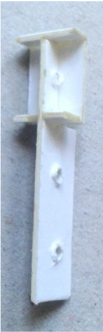
Figure 05.18: Technical development model assembled in stages with new modular joint that bolts to the structure
