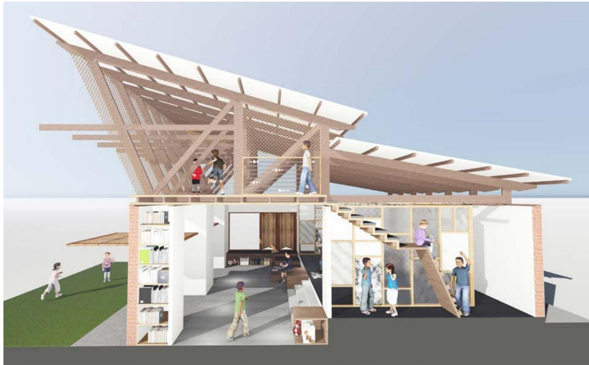
6.10 Section perspective of the contained space showing the habitable wall and roof space. (Author 2017)
