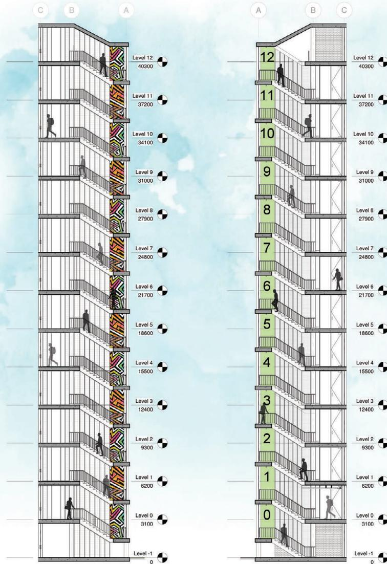
Figure 226 - Section A-A of entire staircase (by Author, not to scale)
