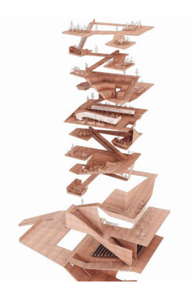
Figure 100 - Model of circulation in building, linking various types of functions easily and as a integrated unit (DS+R 2016)
