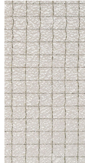
New wired glass glazing Supplier: National Glass Distribution Type: Laminated Georgian Wire Plate Clear Glass Rating: 120 Minutes
