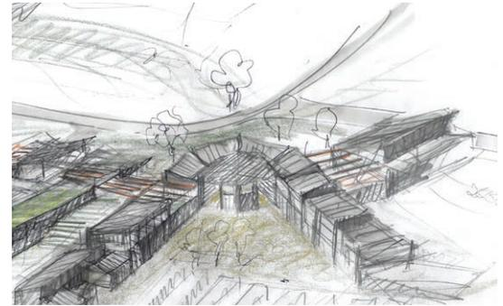
**Figure 3-28:** Above - Iteration 3a & 3b has the public route passing between the northern wing and Champion ring, with a connecting pergola. Iteration 4a changes the orientation of the buildings to face north and has the public route pass diagonally through the building
