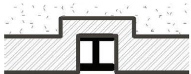
The initial structural system had the columns placed on the outside of a non structural brick skin.
