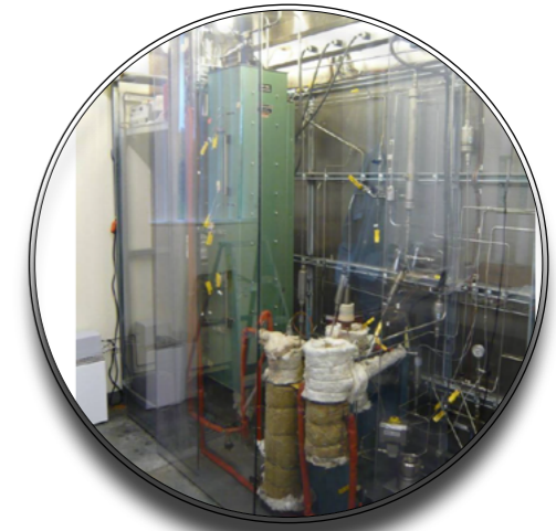
Fig 220: Bench-Scale Oil and Gas System (Old) (Elliot, n.d.)
