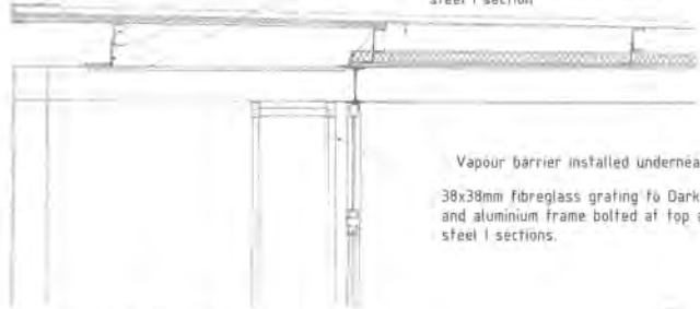
Roof detail Northern facade. NTS
