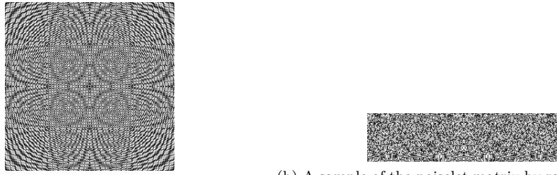
(a) Noiselet matrix with N = 2^8 rows and columns. (b) A sample of the noiselet matrix by randomly picking M < N rows. Figure 3.3.6: The noiselet ensemble.
