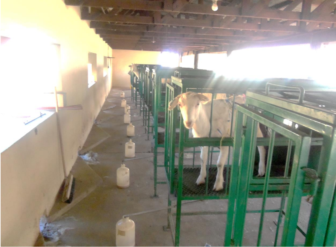
Figure 3.1 Metabolism cages/crates with separate collection of urine
