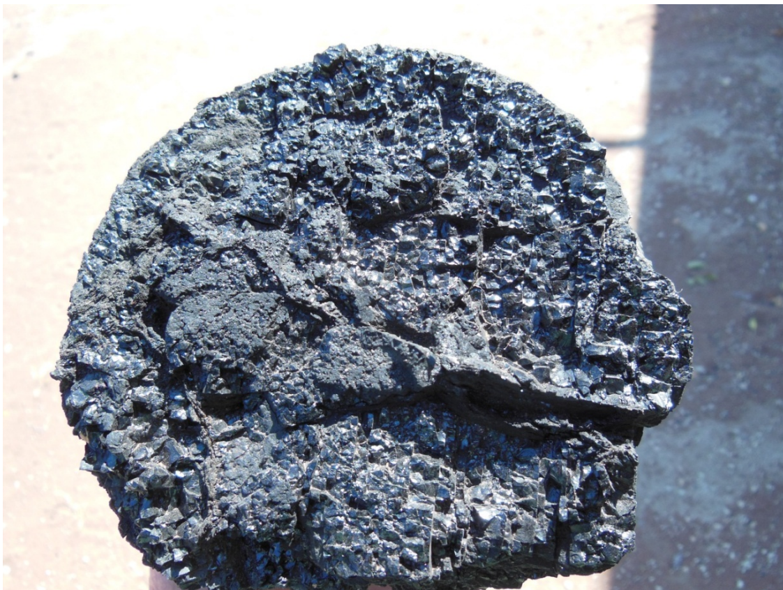
Figure 49: Vitrinite rich coal of the Madzaringwe Formation. Coal cleats can also be seen.
