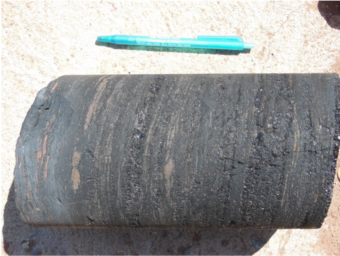
Figure 48: Thinly-laminated coal of the Madzaringwe Formation. Light brown siderite lenses are very common
