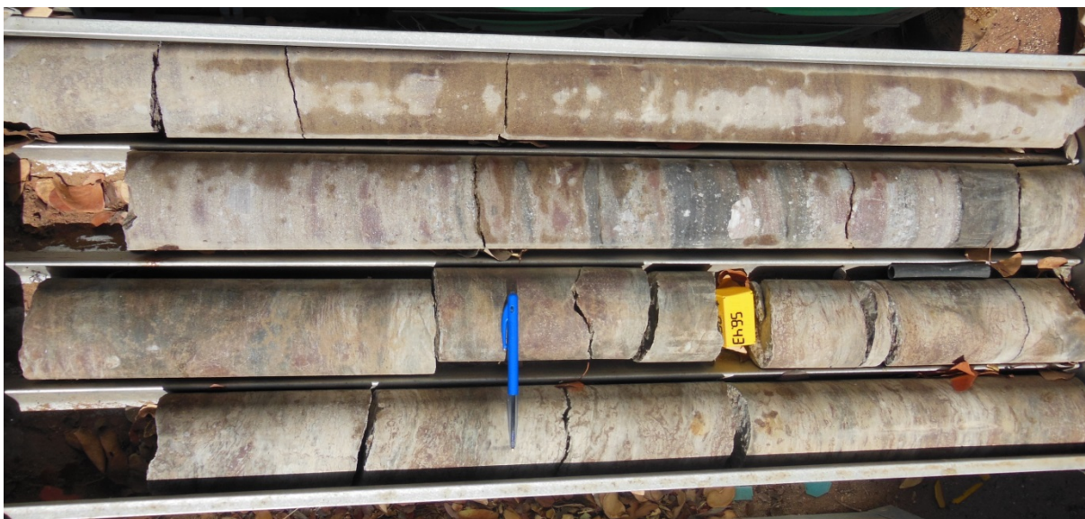
Figure 17: Gradational contact between the basement and the basal arenaceous diamictite unit of the Tshidzi Formation, blue pen is the possible contact.
