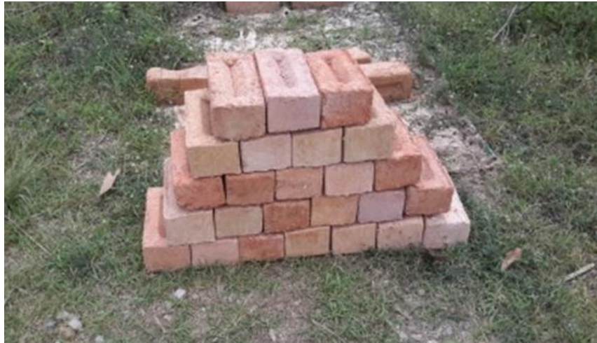
Bricks after 28-day curing, exposed to test for its durability against intense weather, erosion and wind
