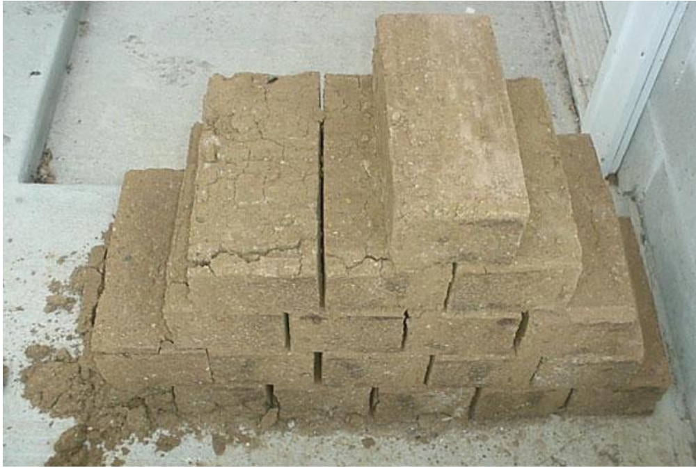
Figure 2.12: Response of compressive earth bricks to climatic conditions after three months
