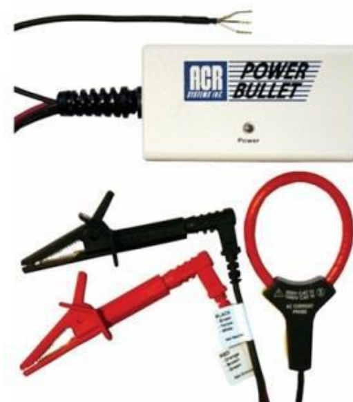
Figure 3.7 Illustration of the energy transducer used during measuring of the grinding energy in the study
