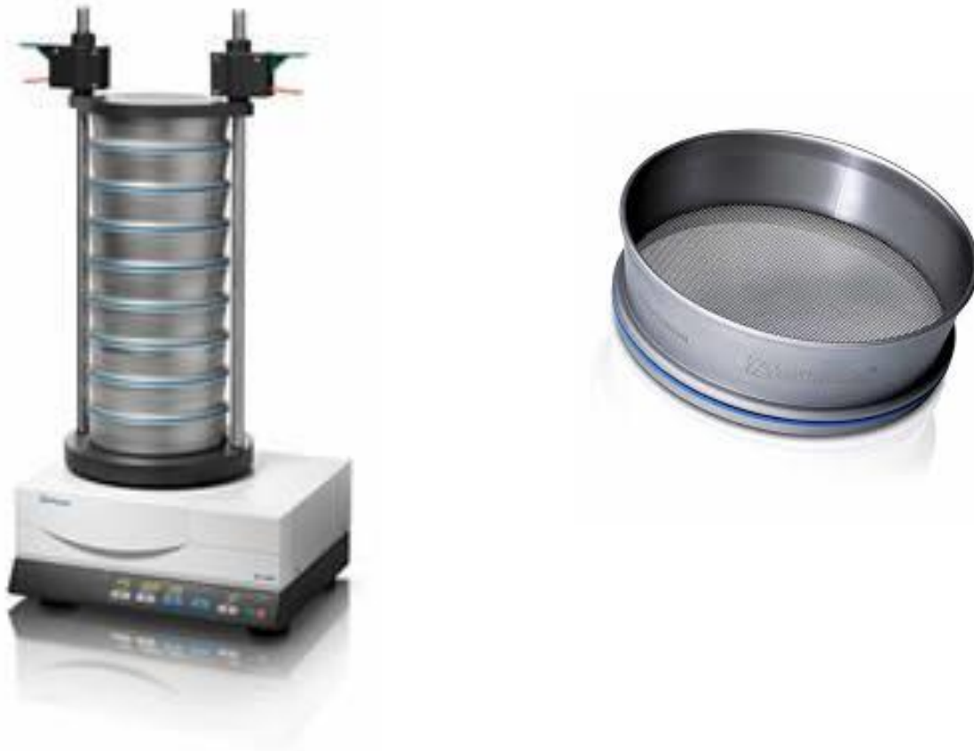
Figure 3.3 Example of Retsch sieve shaker and individual sieve used during the study
