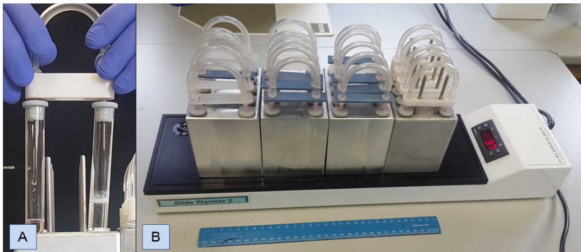
Figure 3.7: A: Connection of culture media and gassing tubes via tubing and needles and B: sets of connected tubes during gas equilibration.
