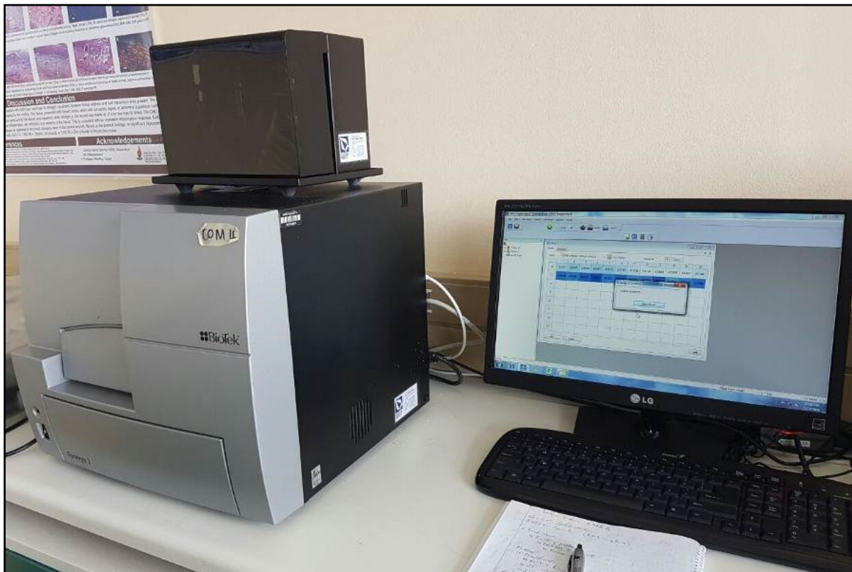
Figure 3.17: Biotek Synergy 2 multimode plate reader used for fluorescence detection to measure the presence of reactive oxygen species.
