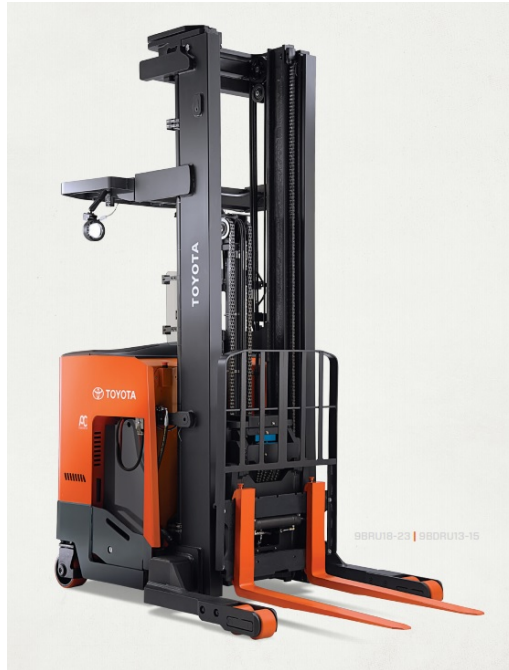
Figure 5.1: Toyota 9BRU18 Reach Truck [Toy]
