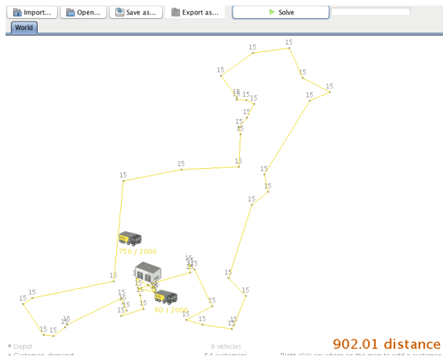
Figure 33: Generated solution for the uncapacitated vehicle routing problem without time windows
