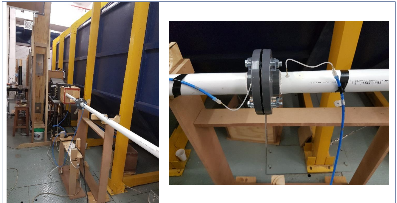
FIGURE 3.14 FILM-COOLING LOOP (LEFT) AND ORIFICE PLATE ASSEMBLY (RIGHT).
