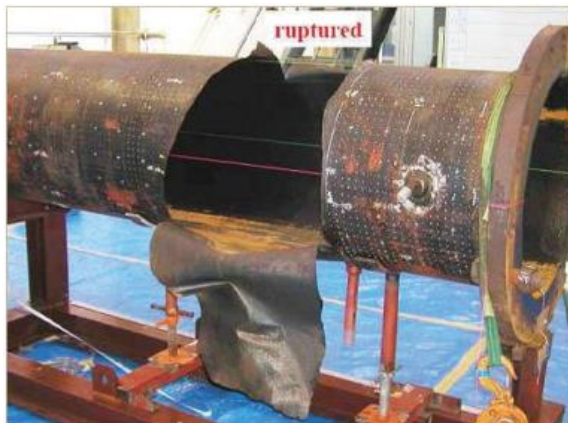
Figure 2: Mihama pressurised water reactor (Uchida 2006)
