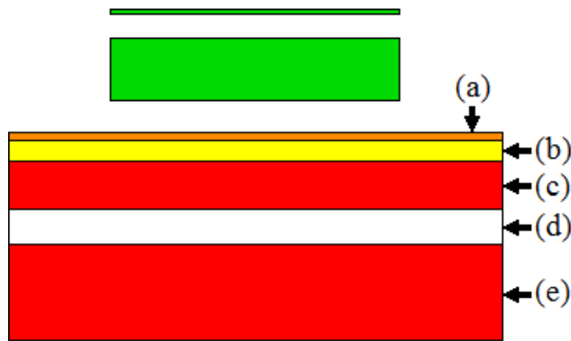
Figure 4.21. Human loading simulation model (the image is not to scale), based on the model from [5]. The antenna is at the top and the simulated human is at the bottom. The width and length of the human tissue model was kept at double that of the antenna. (a) Skin. (b) Fat. (c) Muscle layer 1. (d) Bone. (e) Muscle layer 2.
