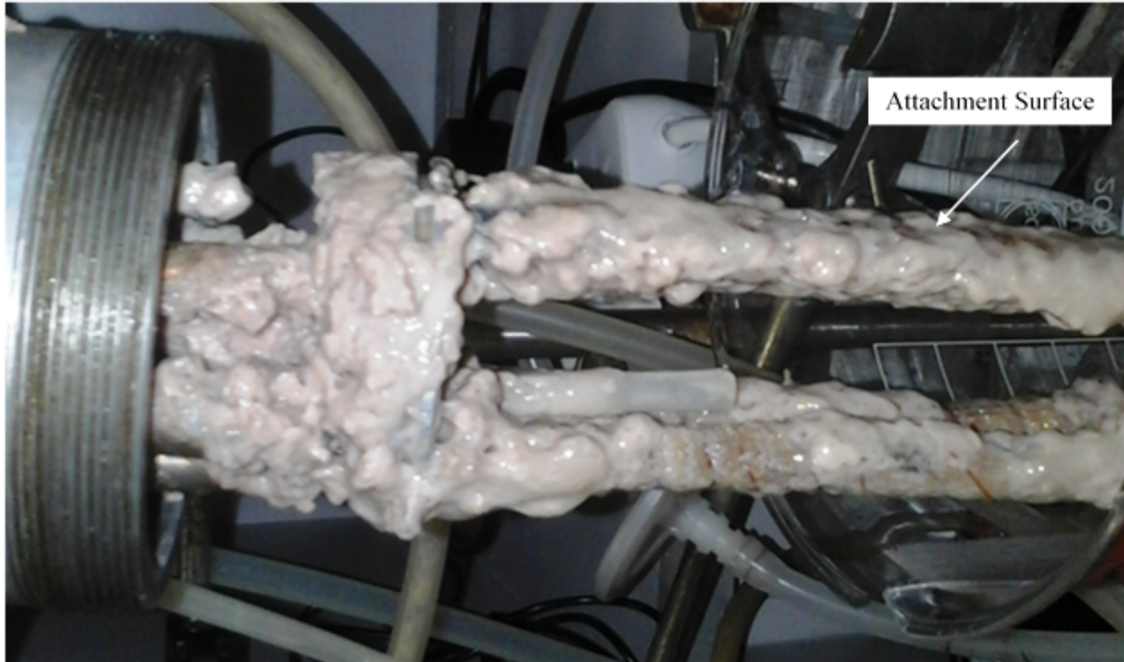
Figure 3.3.5: Biofilm accumulation on the wooden sticks at the termination of the fermentation run.
