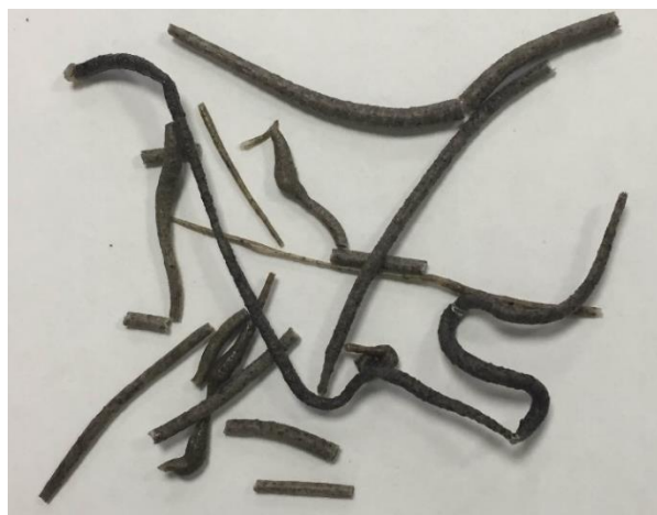
Figure 35: Extruded PCTFE strand showing a large degree of degradation and porous structure
