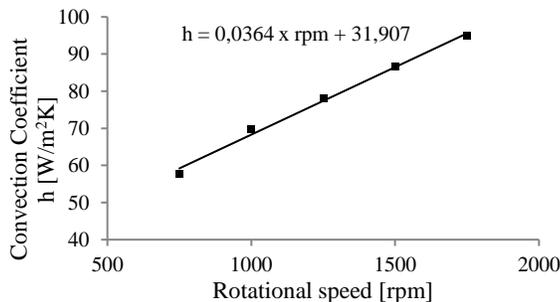
**Figure 6** Convection Coefficient for Ø430 mm size Dry Clutch Pressure Plate
