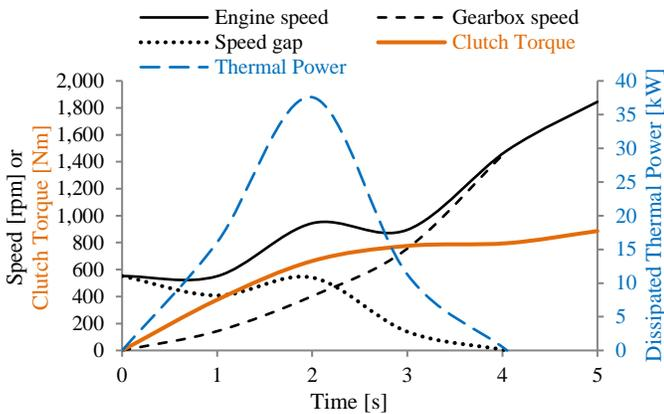
**Figure 2** Speed, Clutch Torque and Dissipated Thermal Power variation during vehicle start-up
