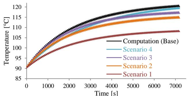
**Figure 8** Pressure Plate mass temperature variation during hill start vehicle test condition
