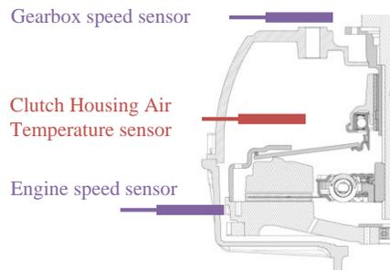
**Figure 3** Sensor instrumentation for hill start vehicle test
