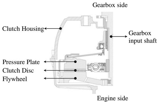
**Figure 1** Dry clutch system
