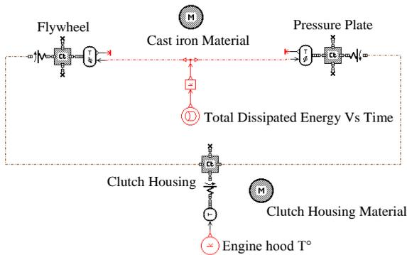
**Figure 5** Schematic view of 1D simulation (Amesim)
