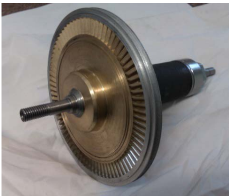
Figure 4 Turbine rotor disk with generator rotor
