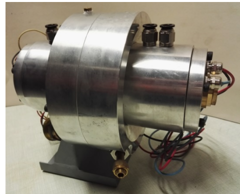
Figure 5 View of microturbine in R-C application
