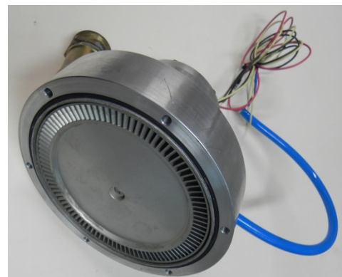
Figure 6 Nozzle disc of microturbine 1st stage
