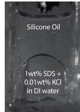
Fig. 3. Electrowetting-controlled single prism module at equilibrium with no voltage applied.
