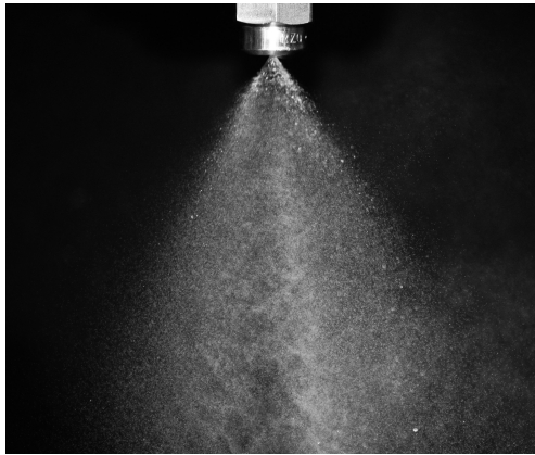
Figure 3. Picture of the spray generated by the atomizer.
