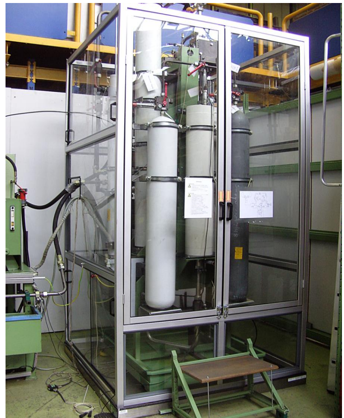
Figure 1 Accumulator Test Set-Up
