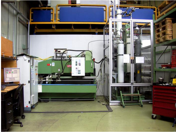
Figure 2 Test-Rig for Experimental Investigations on Hydraulic Devices at Trier University of Applied Sciences
