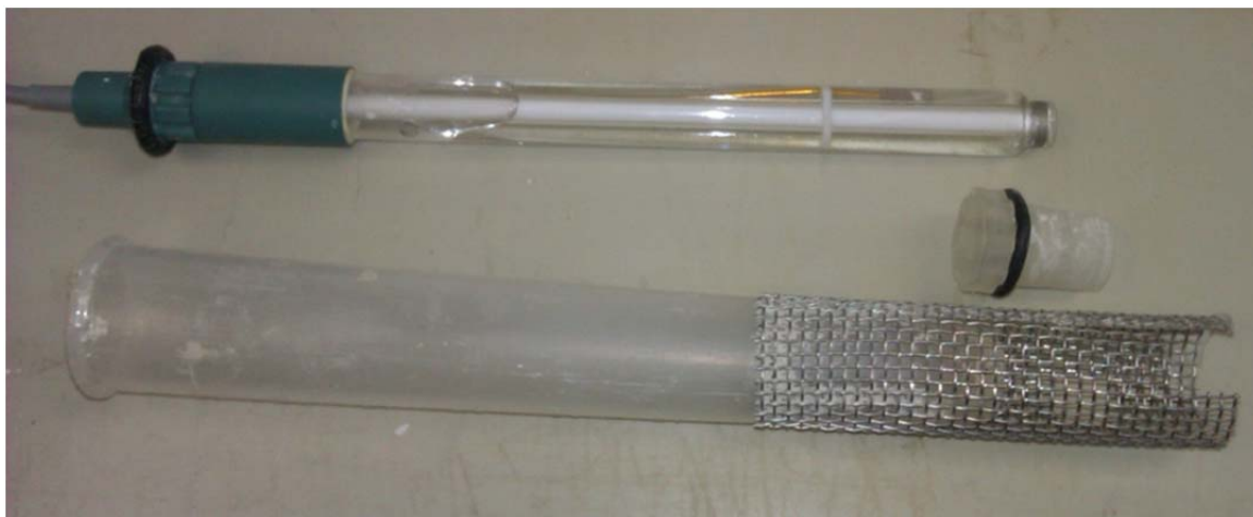
Figure 4. 3: The ORP probe and the probe guard
