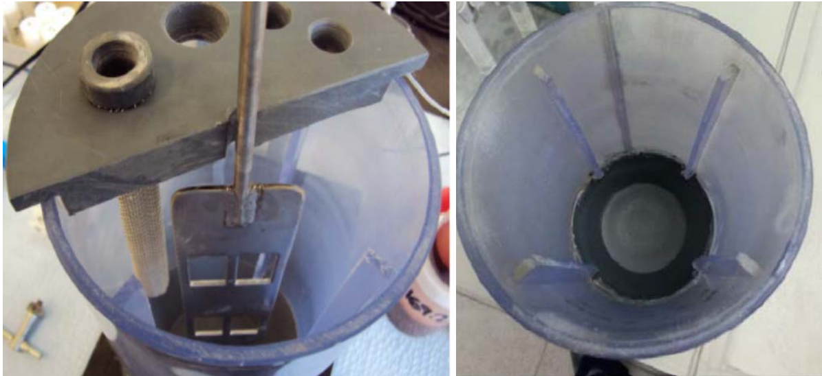
Figure 3. 1: Shows the leach reactor and baffles in leach reactor
