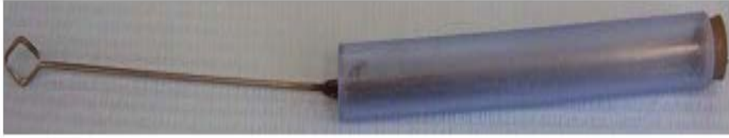
Figure 3. 3: The sampling device used to sub-sample from the vessel during leaching
