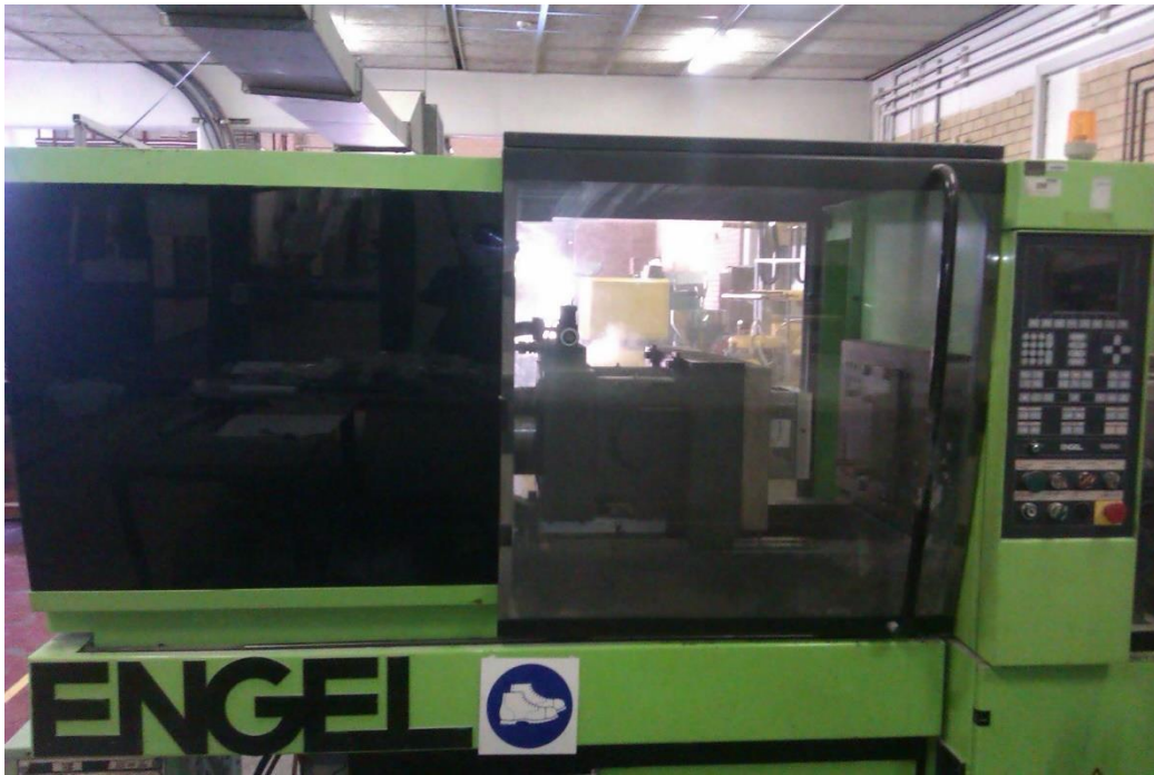
Figure A-8-4: Engel Injection moulder used to make open flame fire testing samples
