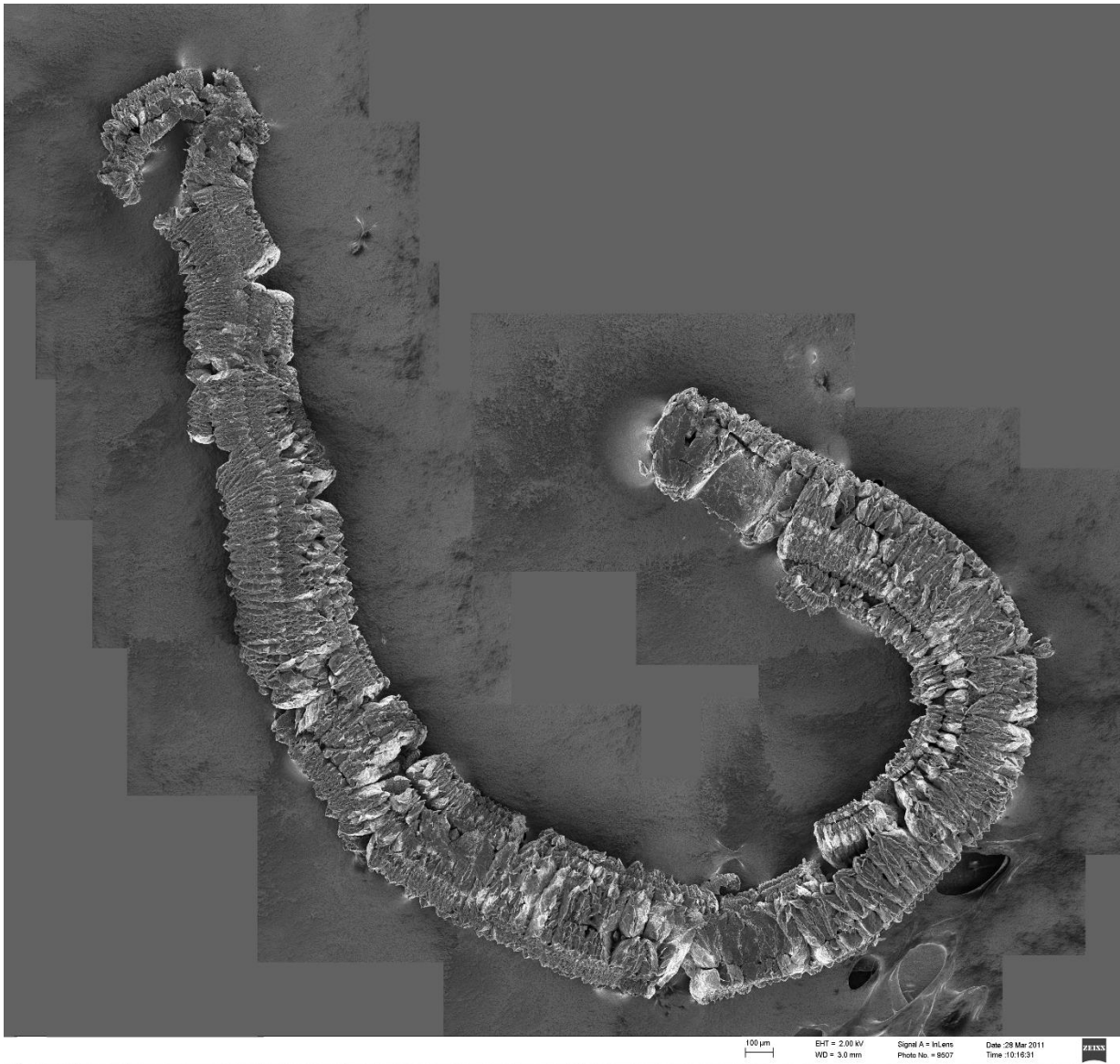
Figure A-2-3: FE SEM micrograph image of ES 250 created by combining multiple micrographs into one image
