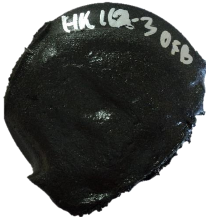
Figure A-8-5: 10% EG 20% DABA sample post exposure to open flame fire testing in the vertical configuration from below
