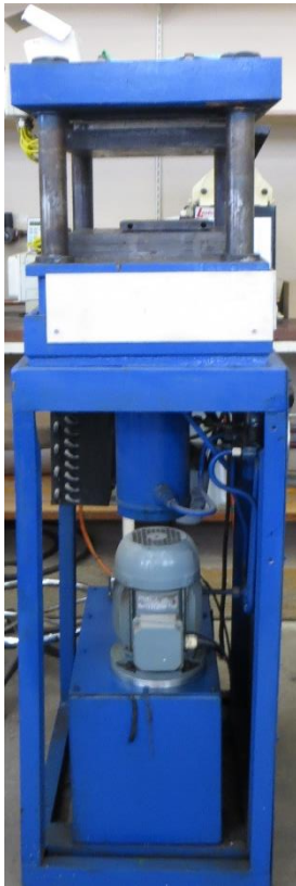
Figure A-8-3: Hot plate press used to prepare the samples used for cone calorimetric testing
