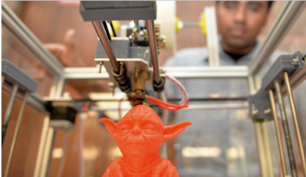
Figure 2.4.1c: 3-D Printed Model Example using a Plastic Material (VanderMey, 2015)
