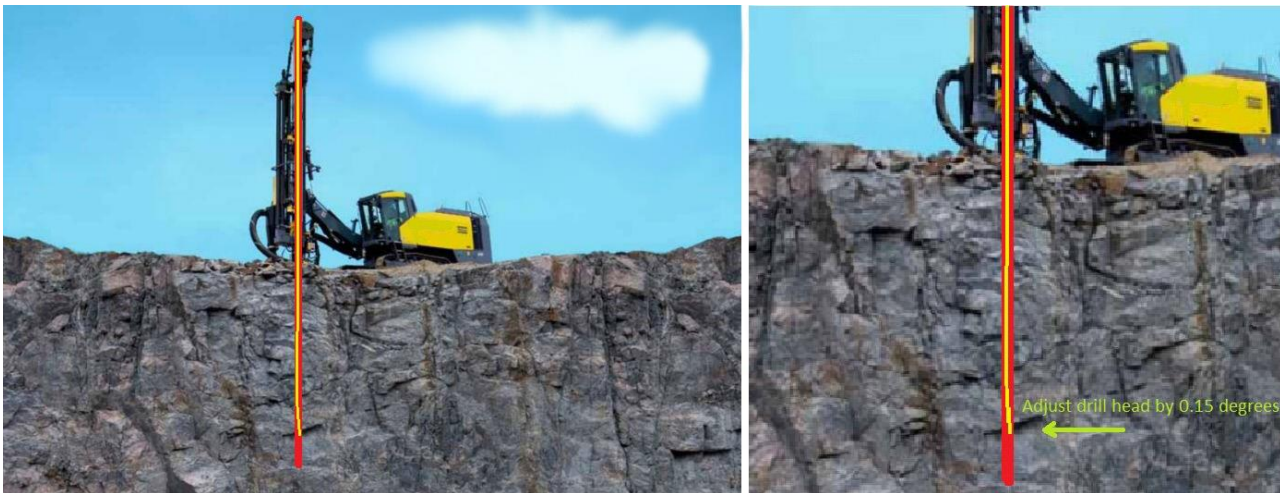
Figure 2.5.5k: Concept for an augmented drill hole with indicated deflection on the drill head (Jacobs, 2015)
