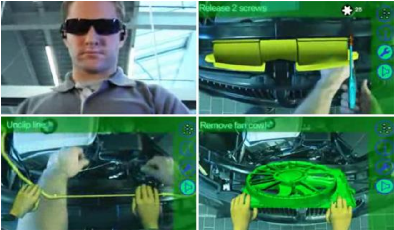
Figure 2.5.5f: BMW uses AR to provide mechanics with step-by-step instructions (Driscoll, 2013)
