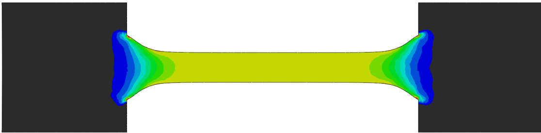
Figure B.5: Final Von Mises stress results of the tensile test for mesh 2 with 1 layer of S4 elements through the thickness for the pre-necking mesh investigation
