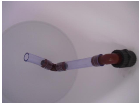
Figure 4.5: Completed plumbing after Being Mounted on the filter bucket
