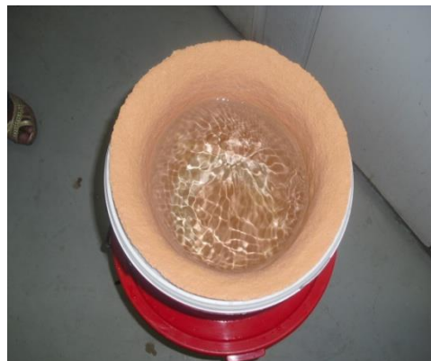
Figure 4.16: Clay pot after being placed in a SIPP receptacle
