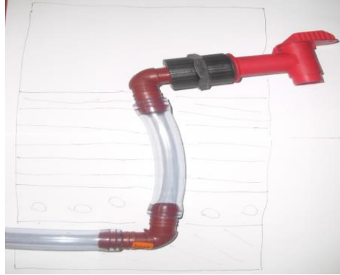
Figure 4.4: Completed plumbing for the BSFZ before being mounted on the filter bucket
