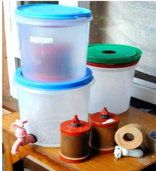
Figure 2.12: Candle filter with ceramic candle filter element (Source: Harvey et al, 2009)
