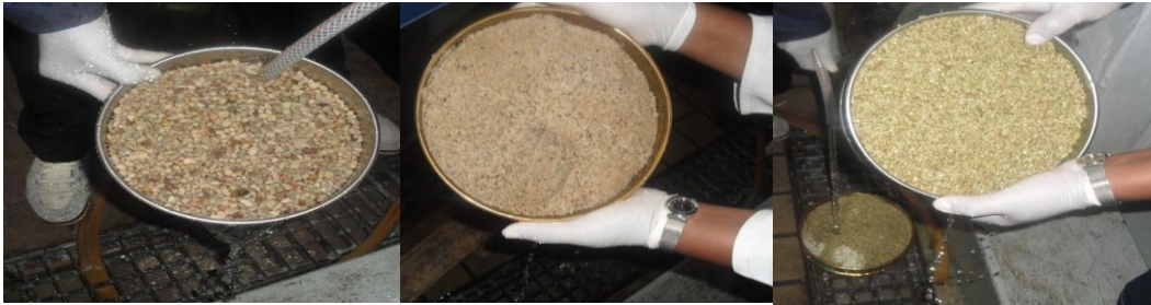
Figure 4.6: Cleaning of the Filter Media with Gravel (left), Coarse Sand (middle) and Zeolites (right)
