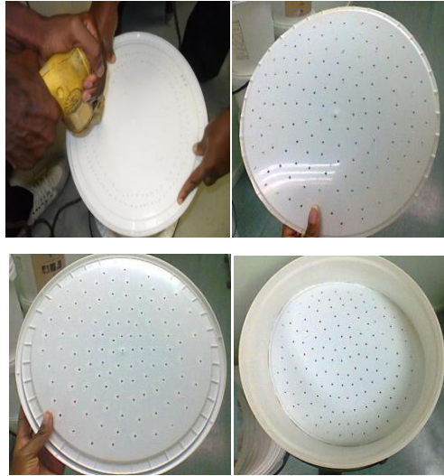
Figure 4.8: Diffusion Plate Construction. Source: Mwabi et al, 2012
