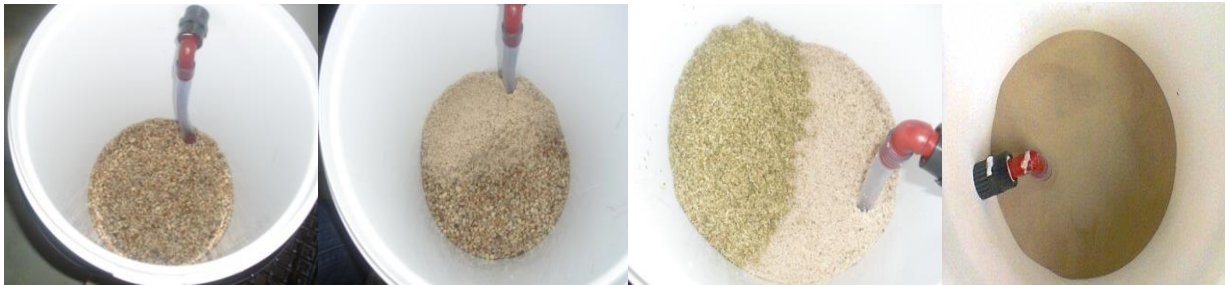
Figure 4.7: Pouring of Filter Media inside the Filter Bucket. Gravel (far left), Coarse Sand (middle left), Zeolites (middle right) and Fine Sand (far right).
