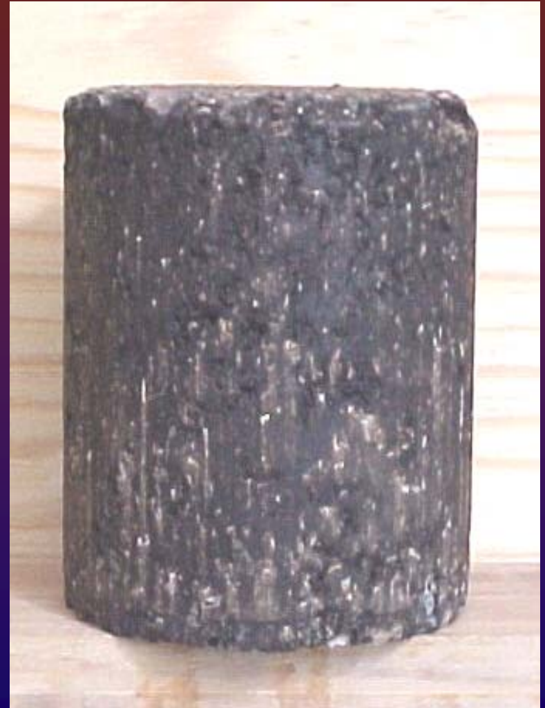
Eroded asphalt sample
