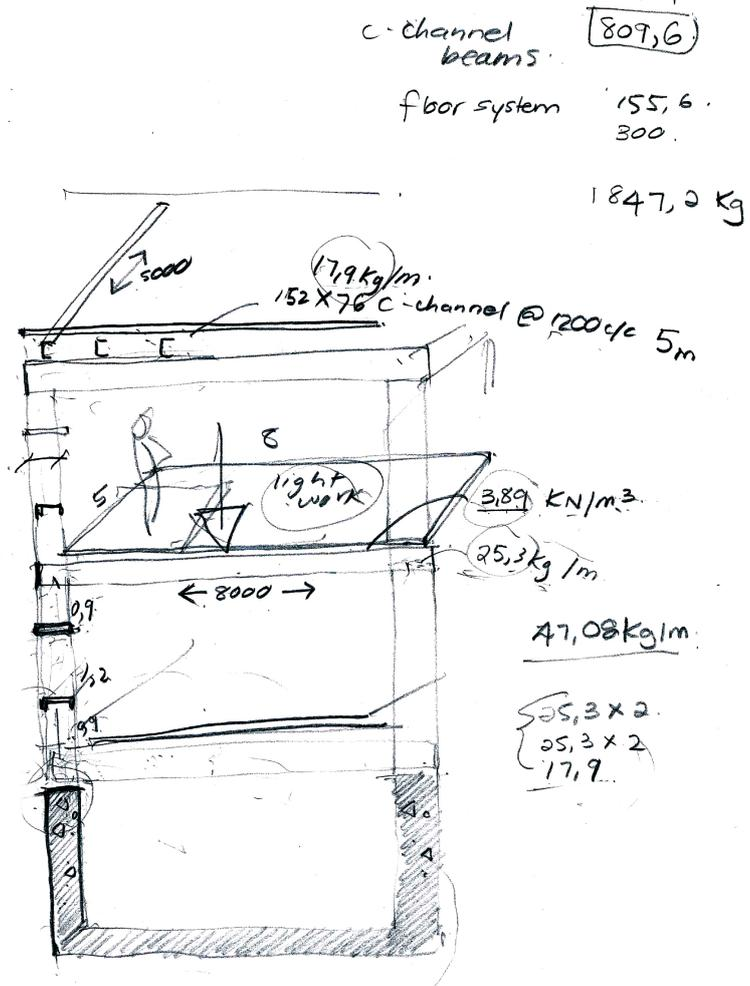
Figure 7.12: Sizing of steel structure. (Author, 2016)
