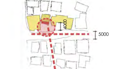
Residential structures often host additional entrepreneurial activities, these are set back from the street forming a courtyard that presents an opportunity for social interaction
