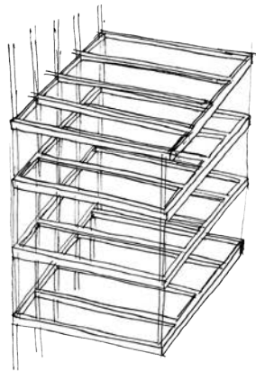
Figure 7.11. Column and beam structure retained and slabs removed (Author 2016)
