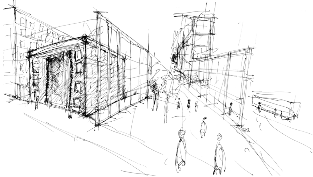
Figure 84 Initial concept sketch for including the heritage building and pushing the proposed building back from the corner.
