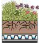
A) Drainage plates Drainage plates are waffled plastic sheets able to store water above and drain water below. They are lightweight, easily installed, and can be specified to meet the water storage requirements of almost any green roof.
