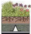
B) Granular Media Lightweight, inorganic, porous granular media is used with triangular drainage conduits. This method is heavier and requires labour intensive installation.
