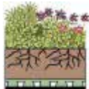
C) Drainage Mats A drainage mat is a layered fabric fulfilling soil separation, drainage, and protection functions. Mats are fast to install and create the thinnest green roof, but have limited water storage and drainage capacity.
