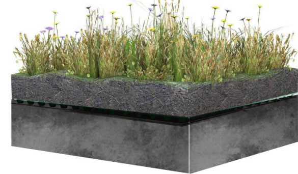
Fig 7.25 Planted concrete roof (Author, June 2016).
