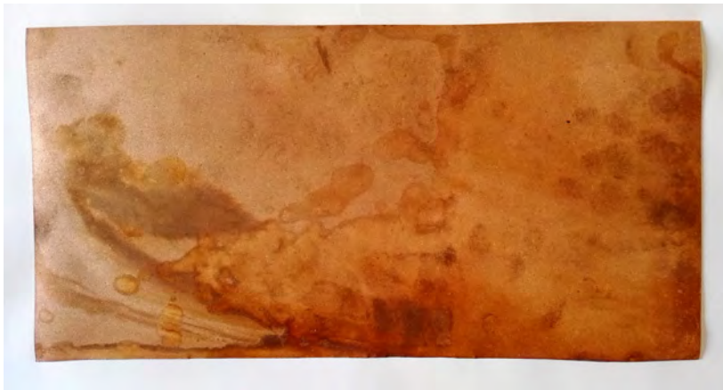
SAND-BLASTED AND DIPPED IN ACID
