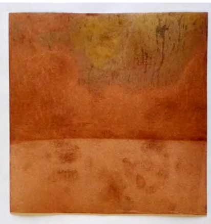
SAND-BLASTED AND PARTIALLY DIPPED IN ACID
