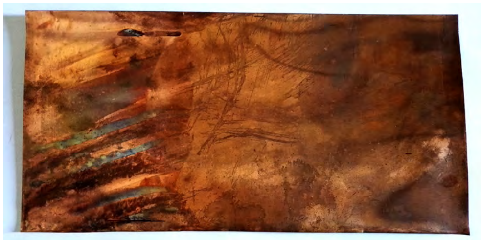
ACID APPLIED USING SPONGE & STEEL WOOL
