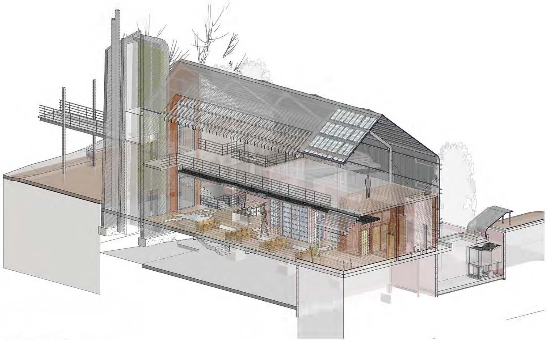
Figure 9.7.3 - Passive ventilation systems
