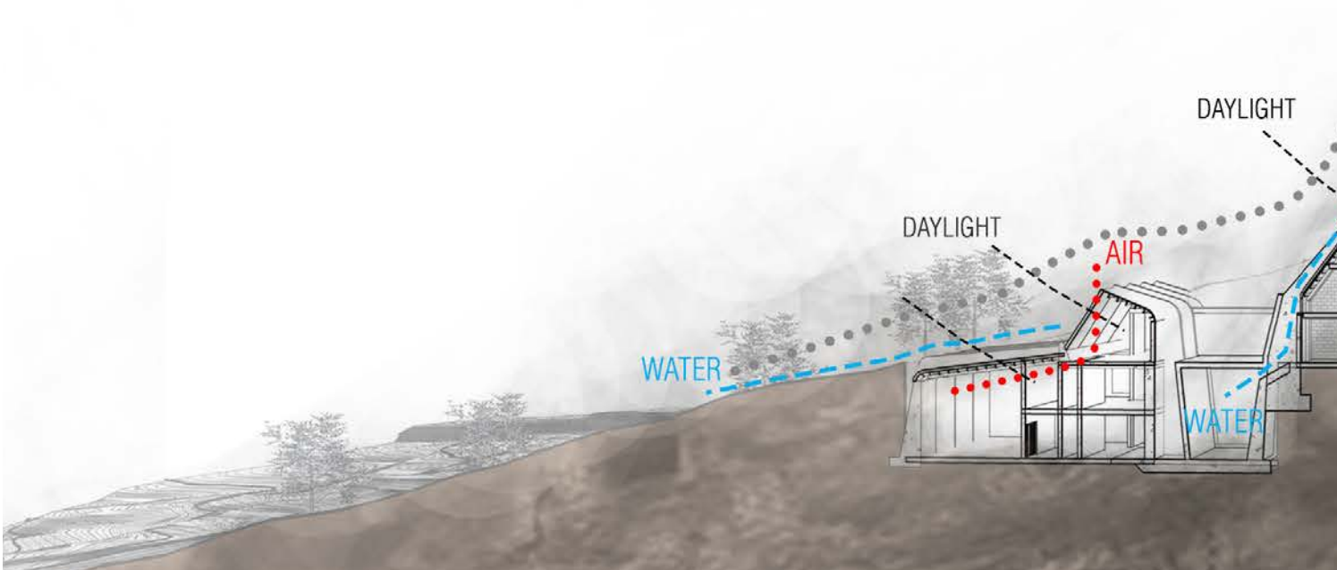
Figure 202: 3-dimensional section of the Workshops and Archive, illustrating how passive strategies were considered. (2016)
