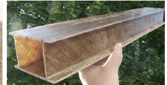
Figure 6.26. Bamboo fiber composite column (Hartford, 2012)
