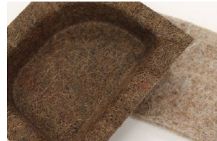
Figure 6.25. Coconut fiber composite (Sharpe, 2013)
