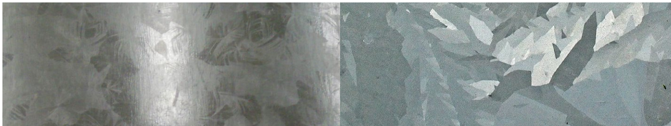
Figure 3.9. Surface Quality of Hot Dipped Metals (ArcelorMittal, 2006)
