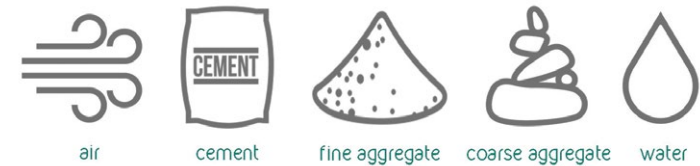
Figure 3.4. Components of Concrete (Author, 2016)
