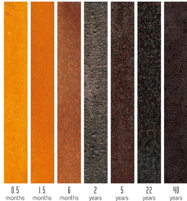
Figure 3.40. COR-TEN Secular Changes in Rust Appearance (Hasegawa, 2016)
