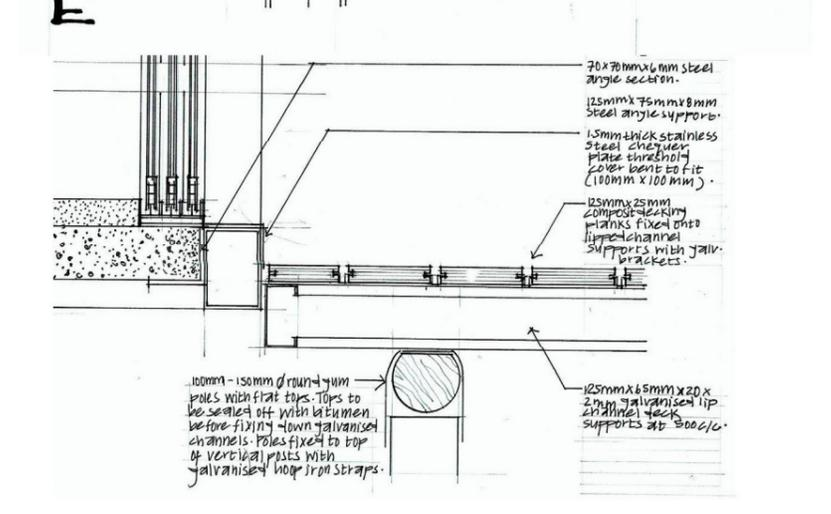
8.5 - Iteration 3, kit assembly system roof details (Author, 2016).
