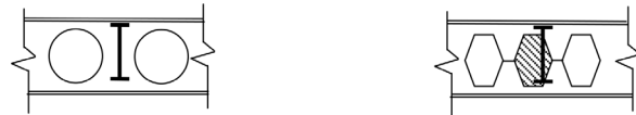
Figure 8.12: Infill plates in castellated beams vs pre-planned cells in cellular beams (Macsteel, n.d)
