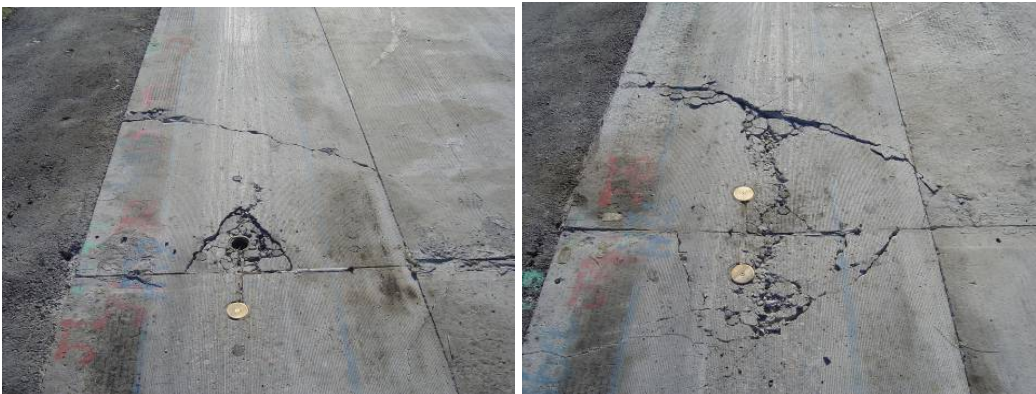
Figure 9. End of life at the two joints of section 1, loaded to failure
