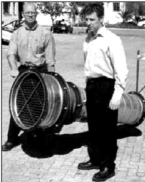
Figure 8: A hydropower venturi air cooler
